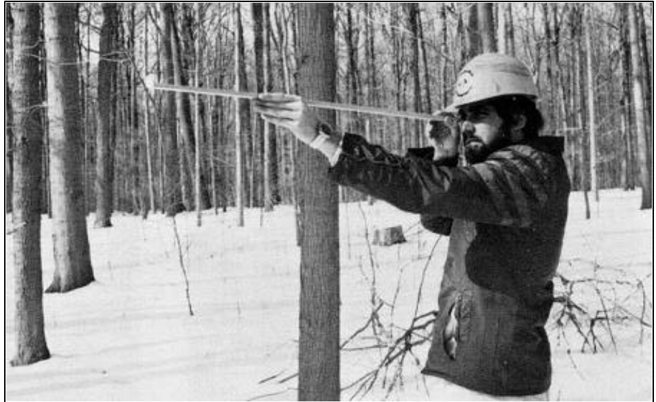
Fig. 4. To estimate basal area using an angle gauge, the observer turns a complete circle over the sampling point and counts the number of tree larger than the width of the block
